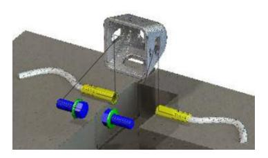
Align prefabricated concrete sections, insert turnbuckle into recess making sure to align anchors to turnbuckle openings.
