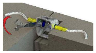
2. The fastener connections are tightened using a ring ratchet wrench until the optimum joint width is reached.
