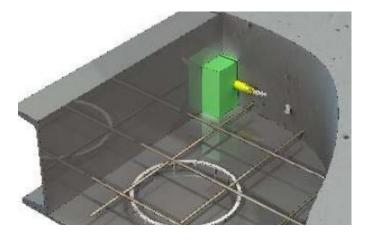
2. Place the recess unit in appropriate position. By marking the formwork and the recess units, the anchors can be precisely fitted with efficiency without extensive measurement.
