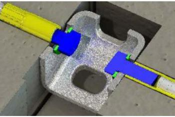
When the prefabricated sections are under tension, the recesses for the tie points can be sealed with appropriate sealing materials and the external recess is ready to be filled.
