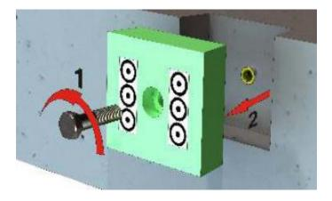
3. After concrete has cured, the recess units are removed leaving open recess in formwork to affix the turnbuckle in place to anchor
